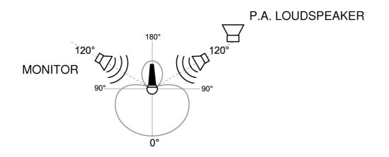
Recommended Loudspeaker Locations for Supercardioid Microphones
