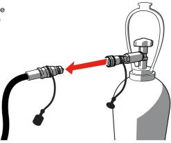
Remove the CO<sub>2</sub> Bottle to Hose Connector from the cylinder.
