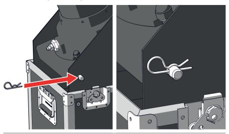
6 Set the angle of the woofer by aligning the back pinhole with one of the four predefined holes in the case.
