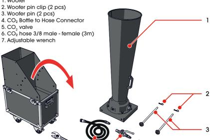
4 Place and hold the woofer in the case and insert a pin through the front pinholes. Make sure that the CO<sub>2</sub> input of the woofer is positioned at the front.
