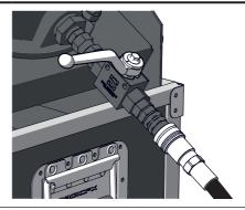
Close the connected CO<sub>2</sub> cylinder.
