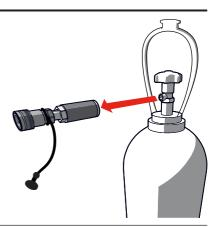
6 Connect a CO<sub>2</sub> Bottle to Hose Connector to a new CO<sub>2</sub> cylinder.
