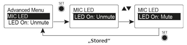
In the **MIC LED** menu item you can configure and deactivate the **STATUS** LED (see "Connecting the RMS 1 mute switch to the SK 300") of the RMS 1 remote mute switch regardless of the settings of the "Advanced > Mute Mode menu item" and the status of the RF signal.
