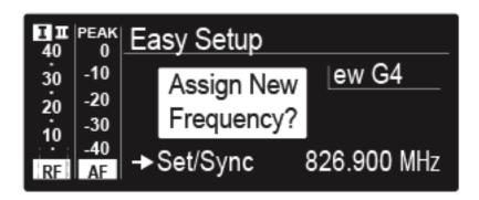
▶ Press the jog dial (SET) on the particular receiver to save your selected frequency and synchronize it with the corresponding transmitter at a later point (see "Synchronizing devices").
