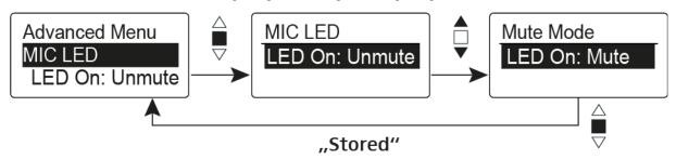
In the **MIC LED** menu item you can configure and deactivate the background lighting of the **MIC** button regardless of the settings of the "Advanced > Mute Mode menu item" and the status of the RF signal.
