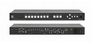
The VP-773 is a high-performance presentation switcher and scaler. It accepts one of eight inputs: one DisplayPort (DP), one composite video, two computer graphics and four HDMI signals. It scales the video, embeds the audio, and simultaneously outputs the signal to two identical HDMI and one HDBaseT TP output, together with S/PDIF and balanced stereo audio outputs.
